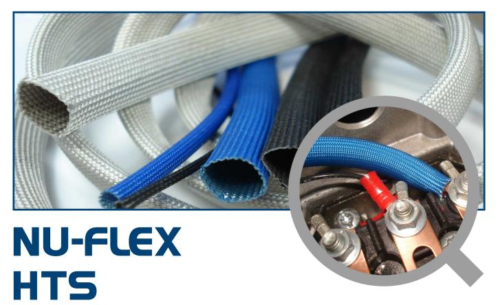
NU-FLEX HTS is a tightly woven, flexible, continuous filament electrical grade 100% fiberglass braid that is heat treated to remove all organic matter and then saturated with an acrylic binder.
